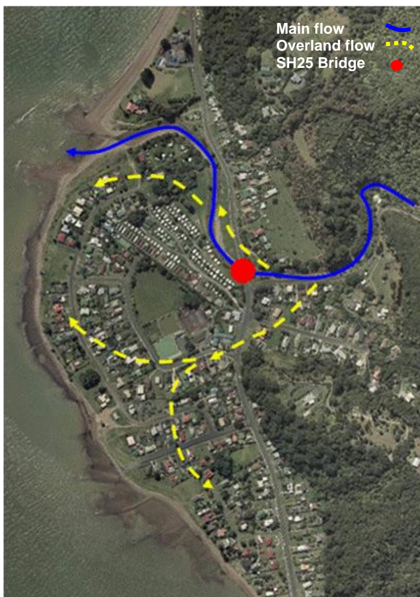
Figure 6 Predominant flooding mechanism at Te Puru
