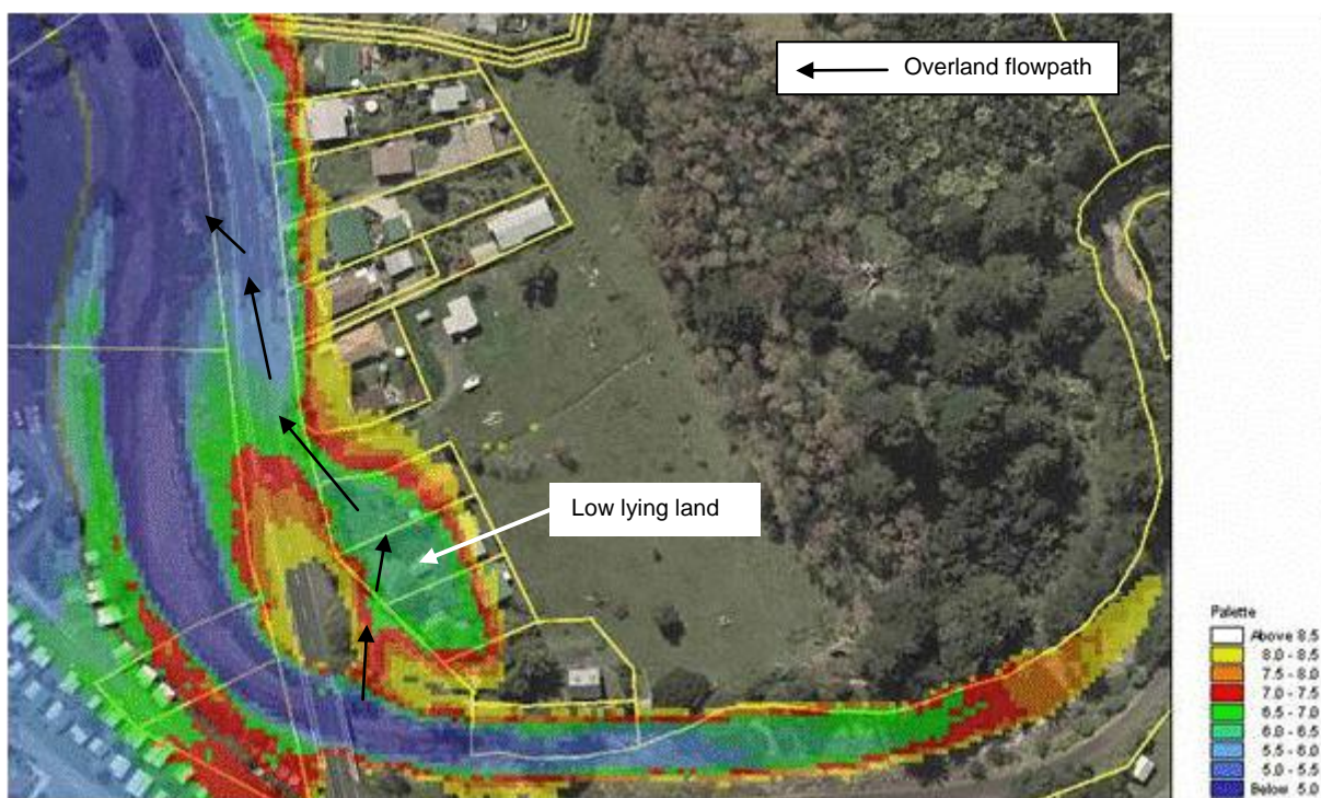
Figure 17 Existing ground levels in the vicinity of the proposed spillway (RL local datum)
